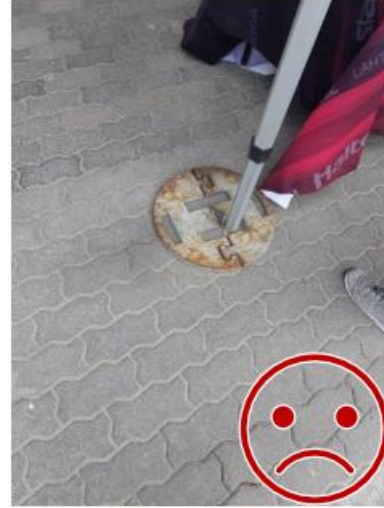
Figure 2. The plate is too small and incompatible with the weight. In this case, a second weight is missing, so the lower weight is not locked in place.
