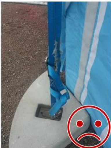
Figure 11. The strap has worn down.
